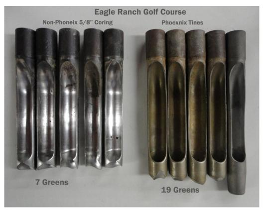
Eagle Ranch Golf Course in Eagle, Colorado used both Phoenix<sup>™</sup> and non-Phoenix<sup>™</sup> 5/8" X 6". Prior to the aerification they 'top-dressed' with a significant sand mix. This led to a situation of significant tine abrasion where the non-Phoenix<sup>™</sup> tines wore out and had to be replaced in just 5-6 greens [40,000 sq. ft.]. The Phoenix<sup>™</sup> treated tines completed all 18 greens and the putting surface and could have done more.
